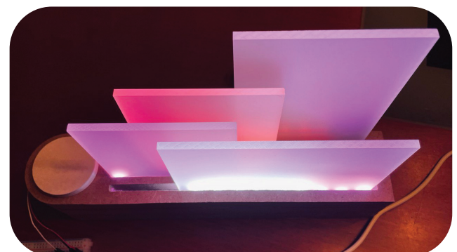
Figure 29. LED's emitting light under frosted perspex glass
